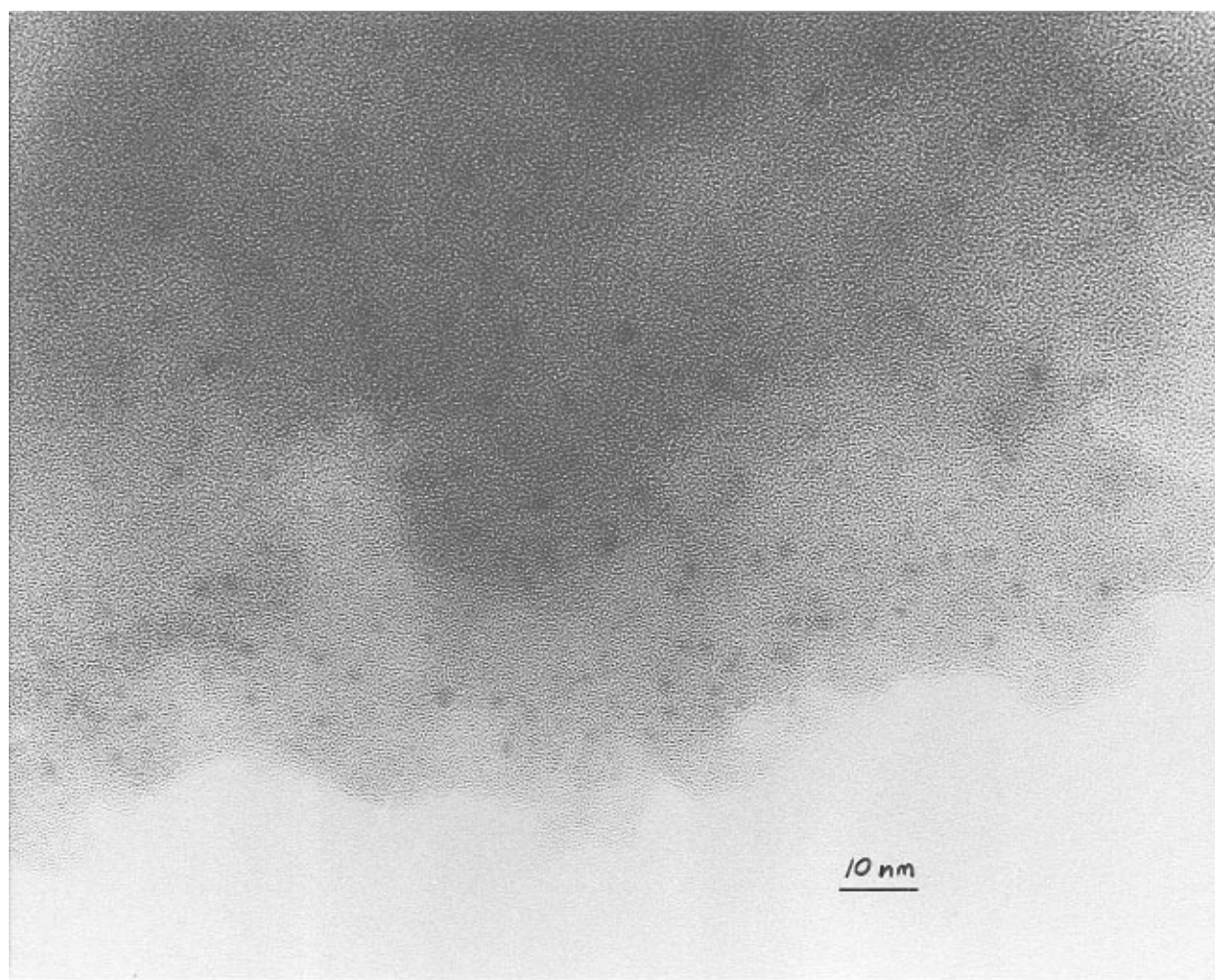
Figure 3. TEM of Au clusters embedded in silica matrix. The particles are 5.7 nm in diameter and highly dispersed. Particle size is roughly twice that of Au clusters synthesized in traditional DDAB/toluene solutions without TEOS. Particle size is independent of gel precursor type, drying procedure, or the \text{H}_2\text{O}:\text{Si} ratio.
